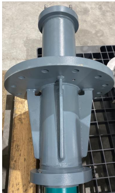
Welding below mounting plate
