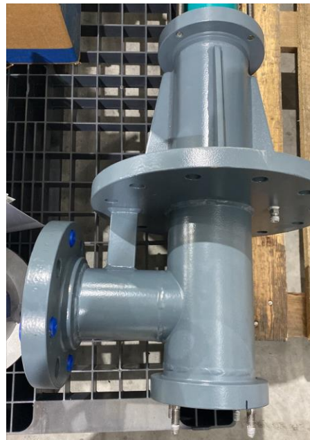
Welding above mounting plate
