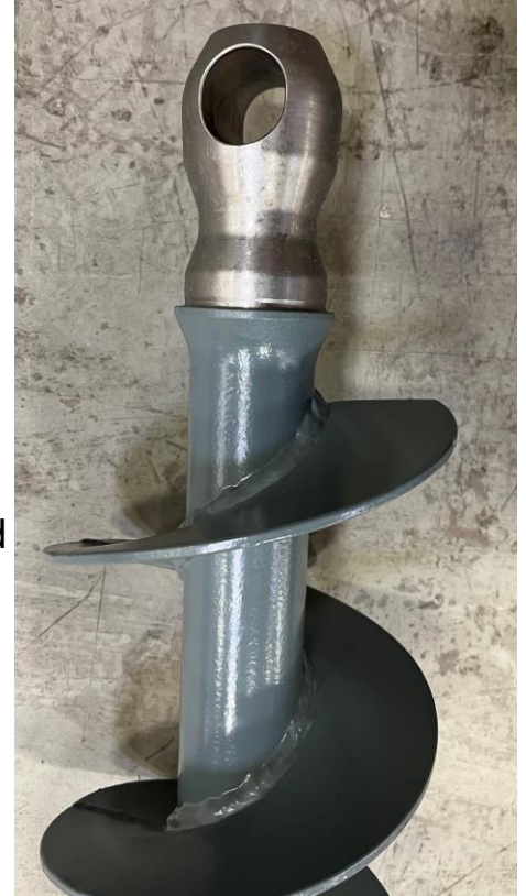
Coupling rod machined
