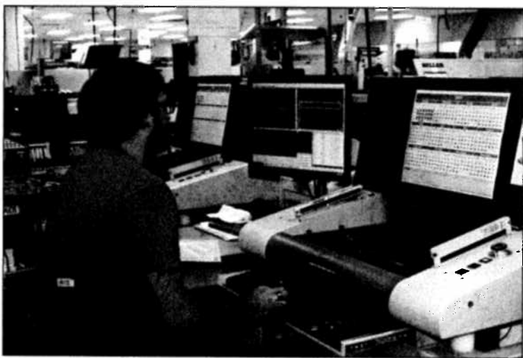
Jason Crook uses an AOI inspection machine to check the quality of circuit boards at Cirtronics Corporation.
